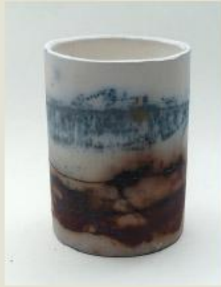
Slipcasting bisque fired to 1050 °C
